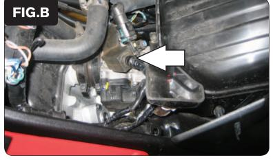
Disconnect the stock connector from the bikes injector, this connector is covered by a rubber boot (Fig B).
