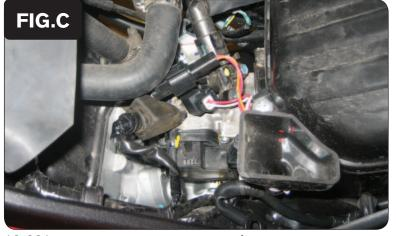
Plug the PCV connectors in-line with the stock harness and injector (Fig C). 5
