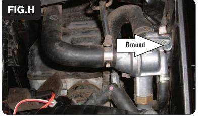
14 Ground the other end of the Dynojet O2 Optimizer to the bolt of the thermostat housing (Fig. H).
