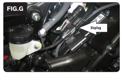
Locate the stock O2 sensor connection on the right side of the bike, over the stock ECU (Fig. G).
