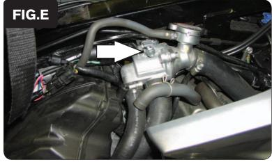
7 To gain access to the #3 and #4 injectors remove the bolts that hold the thermostat to frame. Move the thermostat out of the way temporarily.
