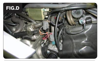
6 Plug the PCV wiring harness in-line of the stock harness and injectors (Fig. D).
