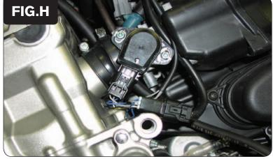
12 Plug the PCV harness in-line of the stock wiring harness and TPS (Fig. H)
