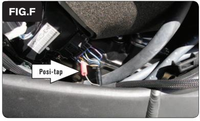
10 Using the supplied posi-tap attach the GREY wire of the PCV to the BLUE/BLACK wire of the stock Throttle Position Sensor harness.
