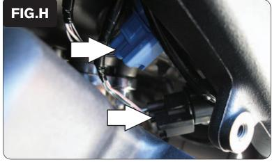
12 Unplug the stock O2 sensors from the stock wiring harness (Fig. H).
