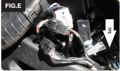
9 Plug the PCV connectors in-line of the stock connectors (Fig. E).
