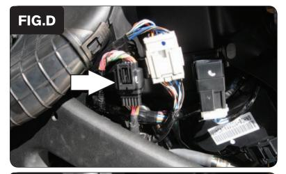
8 Locate the BLACK 12-pin connector on the left side of the airbox (Fig. D). Unplug this connector.
