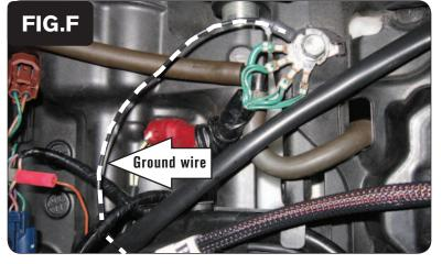
Attach the ground wire from the PCV to the stock common ground location underneath the fuel tank (Fig. F).
