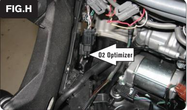
Locate the O2 sensor connection on the left, inside of the frame and unplug this connection (Fig. G).
