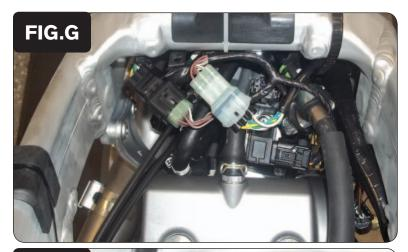
9 Plug the PCV in-line of the stock wiring harness and crank position sensor connector (Fig. G).
