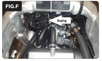
8 Unplug the crank position sensor connector (Fig. F).
