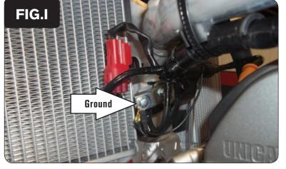
11 Secure the ground wire of the PCV wiring harness with the 6mm ring lug to the stock ground location (Fig. I).
