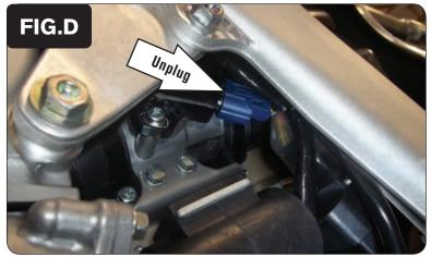
6 Unplug the Throttle Position Sensor harness (Fig. D).
