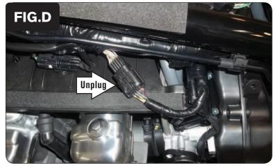
6 Locate and unplug the stock sub-harness connector for the bike's Fuel Injectors (Fig. D).
