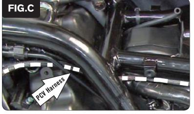
Route the PCV wiring harness forward towards the engine following alongside the stock wiring harness beneath the left side frame rail (Fig. C).
