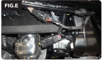
7 Plug the PCV connectors in-line of the stock wiring harness (Fig. E).
