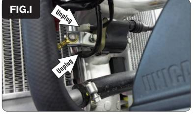
11 Unplug both of the stock coil wires (Fig. I).
