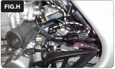
10 Plug the PCV wiring harness in-line of the stock Crank Position Sensor connectors (Fig. H).
