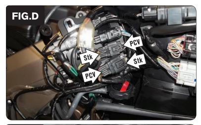
5 Plug the mating pair of 12-pin PCV connectors in-line of the stock fuel injector sub-harness connectors (Fig. D).
