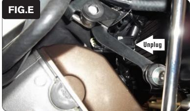
6 Locate and unplug the stock Crank Position Sensor connectors (Fig. E).
