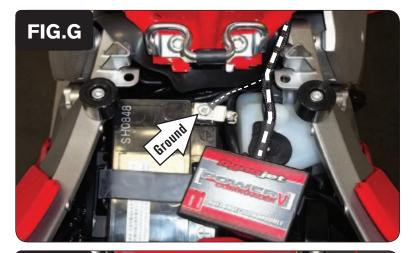
8 Secure the PCV ground wire with the small ring lug to the negative (-) terminal of the bike's battery (Fig. G).
