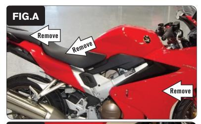
Remove the seats, the plastic panel below the rider's seat that covers the top of the battery, and remove the right and left side mid-fairings (Fig. A).
