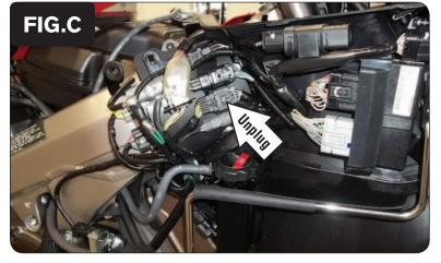
Locate and unplug the stock fuel injector sub-harness connectors (Fig. C).
