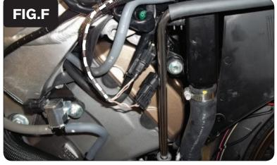
Plug the pair of 2-pin PCV connectors in-line of the stock Crank Position Sensor connectors (Fig. F).
