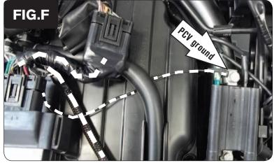
Secure the PCV ground wire with the small ring lug to the right side ignition coil mounting bolt (Fig. F).
