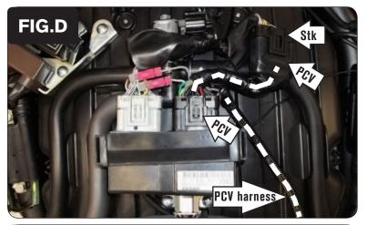
Plug the pair of large connectors of the PCV wiring harness in-line of the bike's ECU and the BLACK stock ECU connector (Fig. D).
