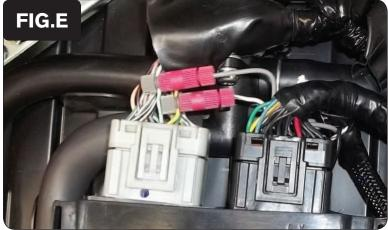
9 Use one of the supplied Posi-taps to attach the PCV unterminated GREY wire to the stock LIGHT BLUE wire of the GREY stock ECU connector.
