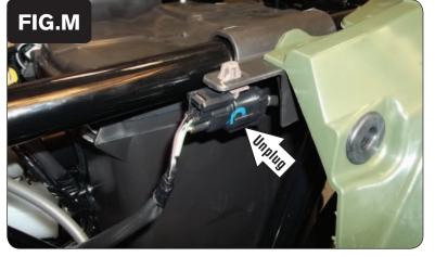
Just left of the airbox, locate and unplug the stock connectors for the ATV's O2 sensor.
