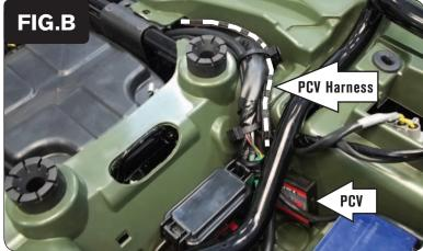
2 Using the supplied Velcro, secure the PCV module to the right side of the compartment directly in front of the battery.
