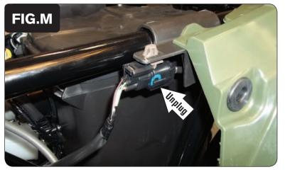
Just left of the airbox, locate and unplug the stock connectors for the ATV's O2 sensor.
