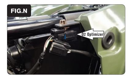
Plug the supplied O2 Optimizer into the ATV's wiring harness in-place of the stock O2 sensor (Fig. N).
