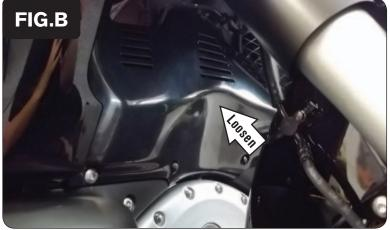
3 Loosen the upper front cowl panel (Fig. B).
