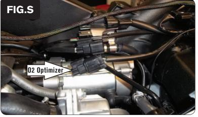
Plug the supplied Right O2 Optimizer (with male pins) into the stock wiring harness in-place of the stock O2 sensor (Fig. S).
