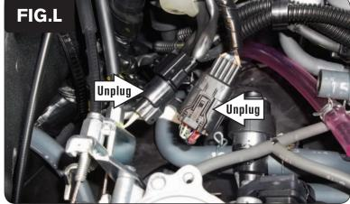
18 Inside of the CLEAR rubber boot just in front of the throttle bodies, locate and unplug the pair of BLACK 10-pin connectors for the bike's left side fuel injectors; and unplug the pair of BLACK 2-pin connectors for the bike's Crank Position Sensor (Fig. L).
