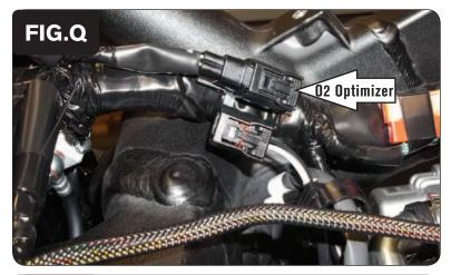
27 Plug the supplied Left O2 Optimizer (with the female pins) into the stock wiring harness in-place of the stock O2 sensor (Fig. Q).
