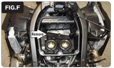
9 Remove the air filter and the air box.
