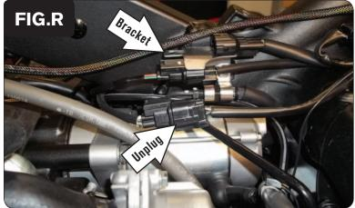
On the right side of the bike just inside the frame and above the starter, locate and unplug the BLACK 4-pin connector for the right O2 sensor that is attached to the metal bracket (Fig. R).
