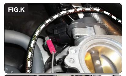
17 Plug the stock TPS connector back on to the TPS (Fig. K).
