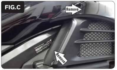
4 Remove the bodywork surrounding the radiators on both sides of the bike (Fig. C).
