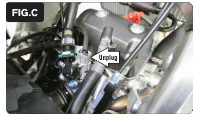
5 Unplug the Fuel Injector (Fig. C).
