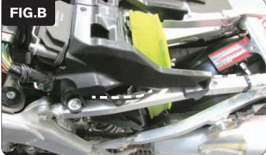
Use the supplied Velcro to secure the PCV module to the top of the rear fender just behind the airbox (Fig. B).
