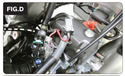
Plug the PCV wiring harness in-line of the Fuel Injector and the stock wiring harness (Fig. D).
