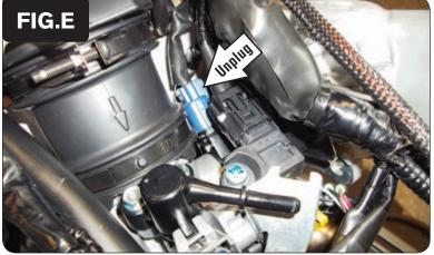
7 Unplug the Throttle Position Sensor at the left side of the throttle body (Fig. E).
