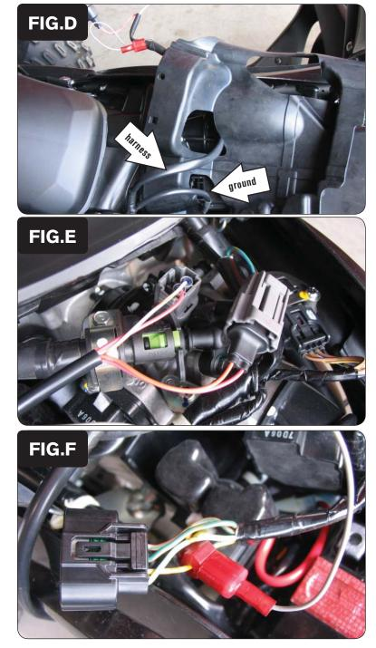
Route the PCFC harness through the rubber cover as shown in Figure D.
