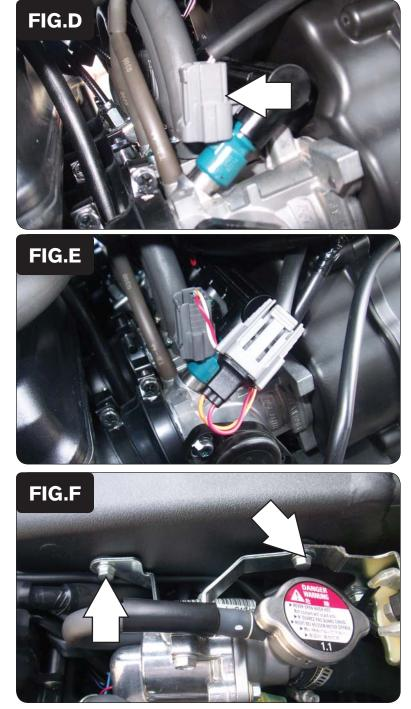
8 Locate the #1 injector connector as shown in Figure D. Unplug this connector.
