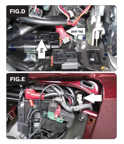
Using the supplied posi-tap, connect the grey wire from the PCFC harness to the red/yellow wire of the stock Throttle Position Sensor (TPS) as shown in Figure D.
