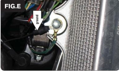
9 Attach the ground wire from the PCFC to the stock ground location as shown in Figure E.
