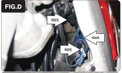
Attach the connectors from the PCFC to the stock TPS connector and the stock wiring harness as shown in Figure D.
