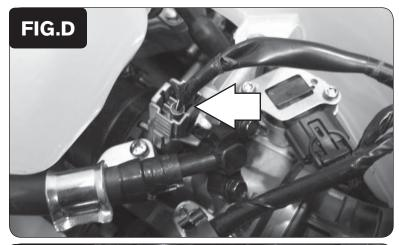
5 Unplug the stock wiring harness from the injector as shown in Figure D.
