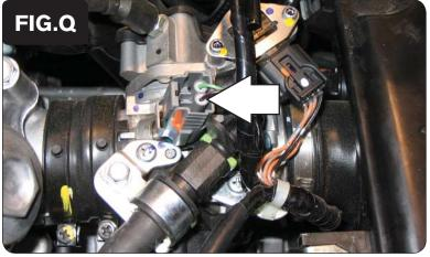
7 Unplug the stock wiring harness from the injector as shown in Figure Q.
