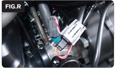
Attach the connectors from the PCFC harness to the injector and stock wiring harness as shown in Figure R.
