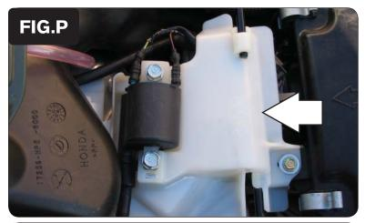
6 Remove the white cover over the throttle body as shown in Figure P.
