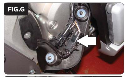
10 Unplug the black 4-pin connector from the O2 sensor as shown in Figure G.
