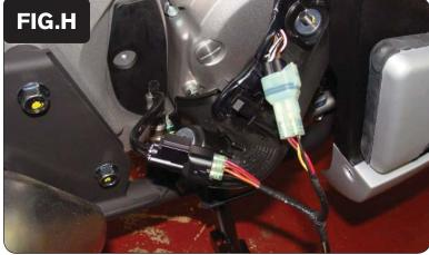
11 Attach the connectors from the PCFC to the stock O2 sensor and wiring harness as shown in Figure H.
