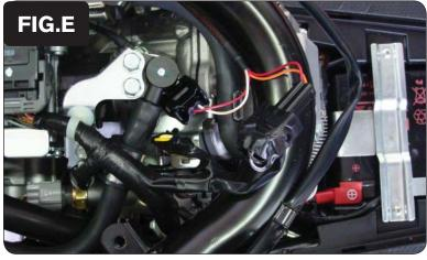
Attach the connectors from the PCFC harness to the stock wiring harness and fuel injector as shown in Figure E.
