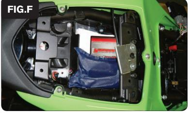
1 Using the supplied velcro, secure the PCV unit in the tail section (Fig. F).
