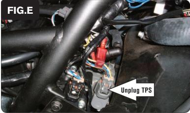
9 Locate the Primary Throttle Position Sensor on the right hand side of the throttle bodies (Fig. E). This is the GREY 3-pin connector.
