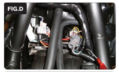
8 Plug the PCV harness in-line of the stock wiring harness and injectors (Fig. D).
