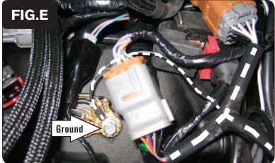
Attach the ground wire from the PCV to the stock wiring harness chassis ground as shown in Figure E.
