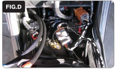
7 Attach the connectors from the PCV to the stock wiring harness and throttle body harness as shown in Figure D.
