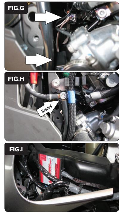
9 Plug the PCV wiring harness in-line of the stock Crank Position Sensor connectors (Fig. G).
