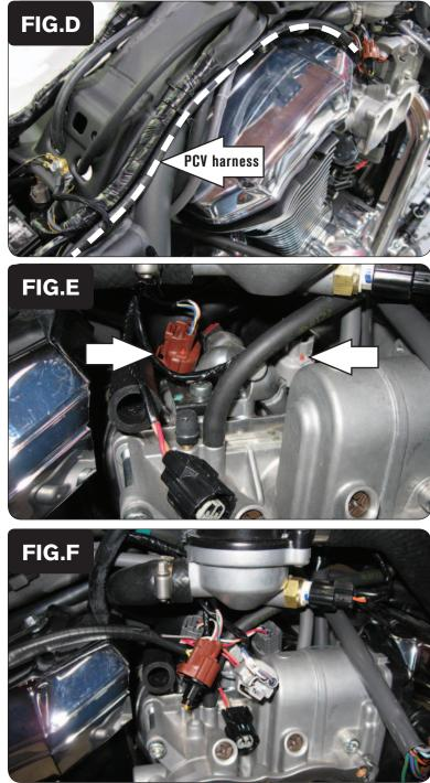
9 Route the PCV harness along the main wiring harness (Fig. D).
