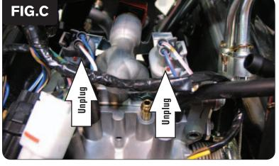
4 Unplug the stock wiring harness from both of the fuel injectors at the top of the throttle bodies (Fig. C).
