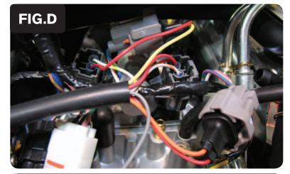
Plug the PCV harness in-line of the stock fuel injectors and the wiring harness (Fig. D).
