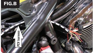
3 Lay the PCV near the battery temporarily. Route the PCV under the frame and route along side the stock harness towards the throttle bodies (Fig. B)
