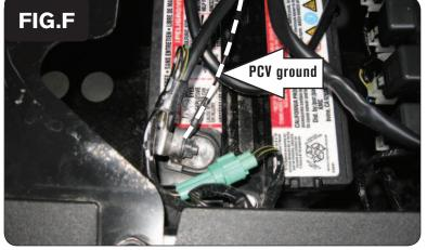
Attach the ground wire from the PCV to the negative side of the battery (Fig. F).
