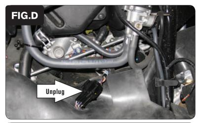
4 Unplug the stock wiring harness from the throttle bodies (Fig. C).
