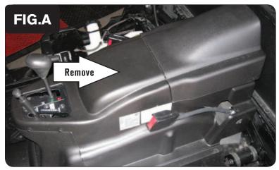
1 Remove the seats. Remove the engine cover (Fig. A).
