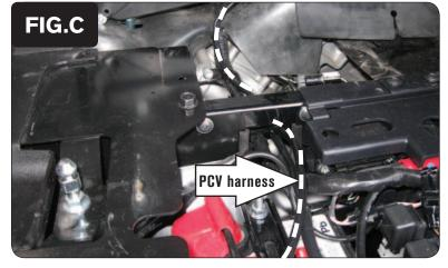
Route the PCV harness from the battery area and go underneath the frame towards the engine (Fig. C)
