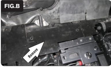
2 Remove the frame cover under the drivers seat by removing the 2 plastic pins (Fig. B)
