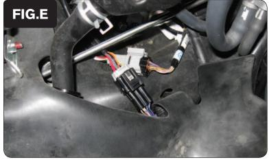
Plug the PCV connectors in-line of the stock wiring harness and throttle body harness (Fig. E).
