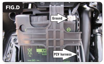
Attach the ground wire from the PCV to the negative side of the battery (Fig. D).
