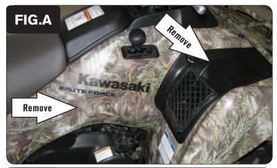
1 Remove the seat. Remove the right hand side cover (Fig. A).
