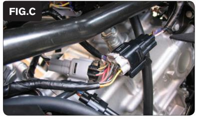
Plug the PCV wiring harness in-line of the stock wiring harness and throttle body harness (Fig. C).
