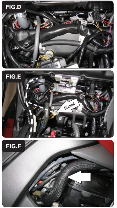
Plug the PCV wiring harness in-line of the stock harness and injectors (Fig. C).PCV harness:
