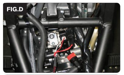
11 Plug the PCV harness in-line of the stock injector and wiring harness (Fig. D).
