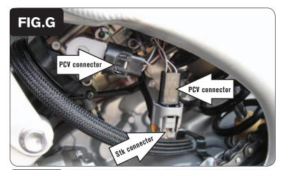
10 Plug the PCV connectors in-line of the stock wiring harness and throttle body (Fig. G).
