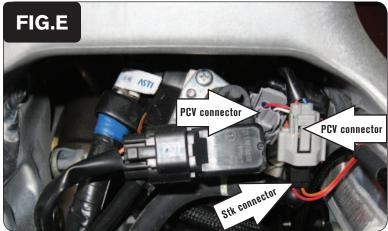
Plug the PCV connectors in-line of the stock wiring harness and fuel injector (Fig. E).
