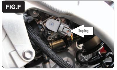
Unplug the stock wiring harness from the Throttle Position Sensor (Fig. F). 9 This connector is located on the left side of the throttle body.
