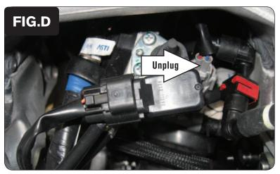
Unplug the stock wiring harness from the injector (Fig. D).
