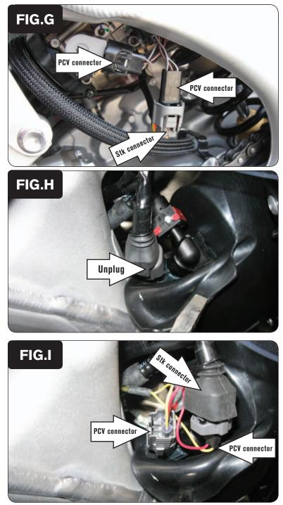
10 Plug the PCV connectors in-line of the stock wiring harness and the Throttle Position Sensor (Fig. G).
