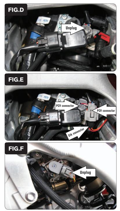
7 Unplug the stock wiring harness from the primary injector (Fig. D).
