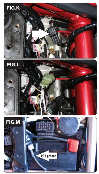
15 Locate the Crank Position Sensor connector to the right rear of the air box (Fig. K).
