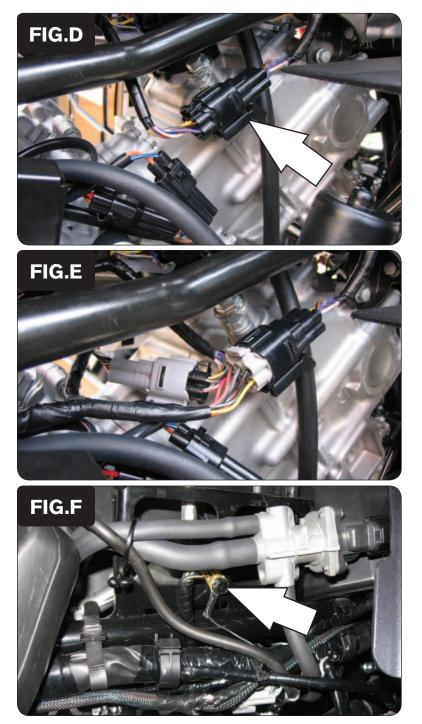
4 Locate the 6-pin BLACK connector that comes from the throttle bodies. Unplug this connector (Fig. D).
