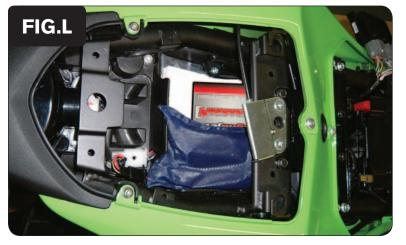
19 Using the supplied velcro, secure the PCV unit in the tail section (Fig. F).
