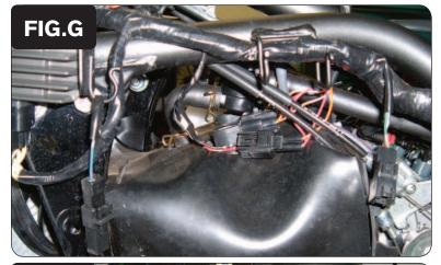
12 Connect PCV in-line of the stock wiring harness and each coil stick.
