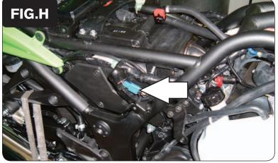
13 Unplug the Crank Position Sensor from the stock wiring harness (Fig. H).
