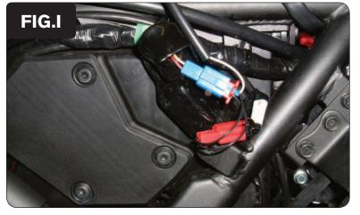
14 Plug the PCV in-line of the stock wiring harness and CPS (Fig. I).
