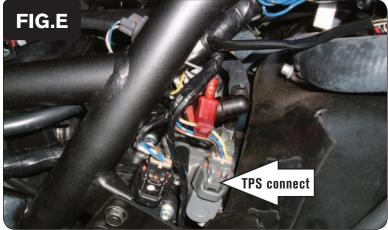
9 Locate the Throttle Position Sensor on the right hand side of the throttle bodies (Fig. E). This is the GREY 3-pin connector
