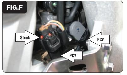
9 Plug the PCV connectors in-line with the ATV's throttle position sensor and stock wiring harness (Fig. F).
