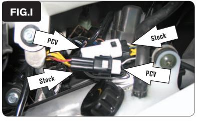
13 Connect the PCV harness in-line of the stock crank position sensor connectors (Fig. I).
