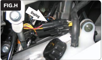
12 Locate and unplug the crank position sensor connector (Fig. H).
