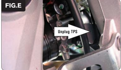
8 Locate the stock throttle position sensor connector on the left hand side of the throttle body. Unplug the stock wiring harness from the TPS (Fig. E).
