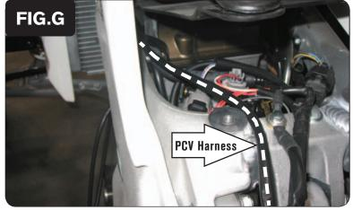
Route the remainder of the PCV harness underneath the fuel tank along the left hand side of the frame (Fig. G).
