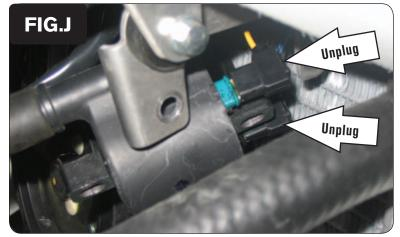
14 Unplug the stock wiring harness from the ignition coil (Fig. J).
