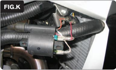
15 Plug the PCV harness in-line of the stock wiring harness and ignition coil.
