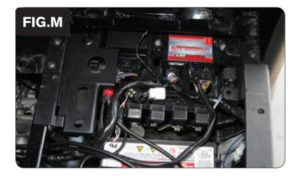
17 Using the supplied velcro secure the PCV module to the top of the ECU (Fig. M).
