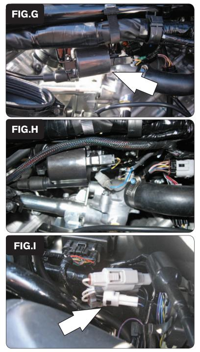
7 Locate the rear ignition coil. It is located on the right hand side of the ATV near the frame rail (Fig. G).
