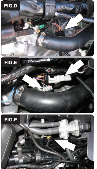
4 Locate the 6-pin BLACK connector on the front head, that comes from the throttle bodies. Unplug this connector (Fig. D).
