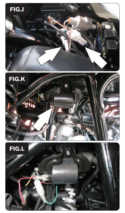
11 Plug the set of WHITE 2-pin connectors of the PCV harness in line with the ATV's crank position sensor connectors (Fig. J).
