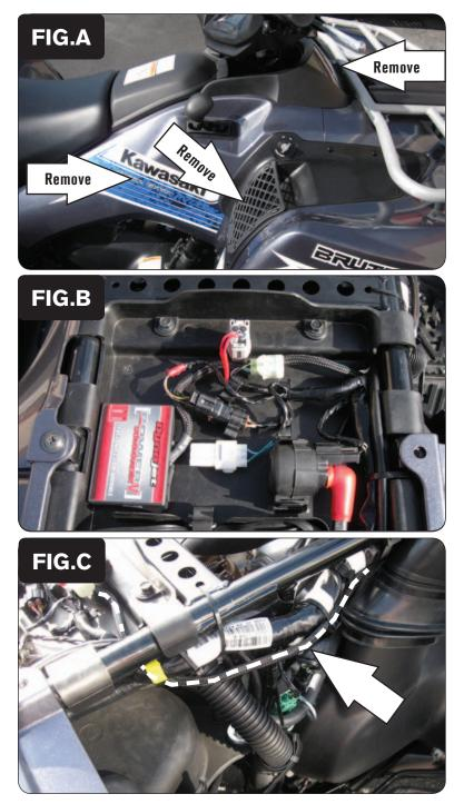
Remove the seat. Remove the right hand side cover, and the cover in front of the steering stem that holds the accessory outlet (Fig. A).
