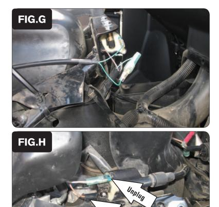
10 Plug the GREEN colored wires of the PCV wiring harness in-line of the GREEN Front Ignition Coil pin and the stock GREEN Front Ignition Coil wire with the CLEAR insulator (Fig. G).
