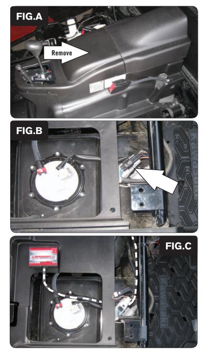
Remove both of the front seats and the engine cover (Fig. A).
