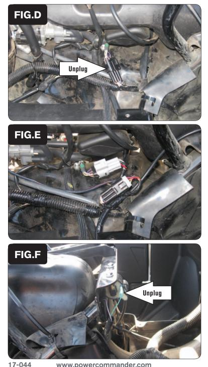
6 Locate and unplug the stock wiring harness from the throttle bodies (Fig. D). This is a BLACK 6-pin connector located at the right side of the engine.
