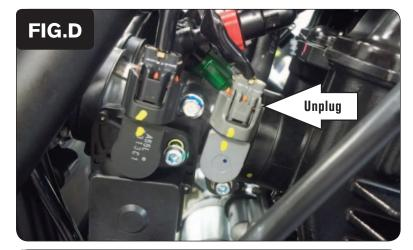
10 Locate the Throttle Position Sensor on the right hand side of the throttle bodies (Fig. D).
