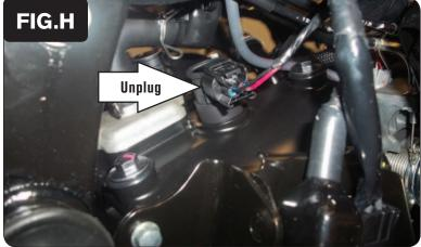
14 Unplug the stock wiring harness from the left ignition coil stick (coil stick #1) (Fig. H).
