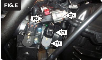
11 Plug the connectors from the PCV wiring harness in-line of the TPS and the stock wiring harness (Fig. E).
