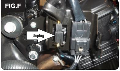
Locate and unplug the Crank Position Sensor from the stock wiring harness (Fig. F).
