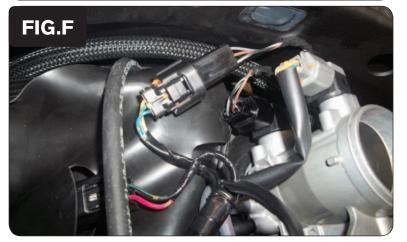
9 Plug the PCV wiring harness in-line of the fuel injector and the stock wiring harness (Fig. D).
