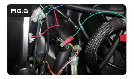
12 Use the supplied Posi-tap to attach the BLUE/ WHITE wire of the PCV wiring harness to the stock GREEN/RED wire of the bike's Gear Position Sensor (Fig. G).
