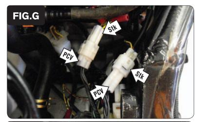
9 Plug the pair of matching PCV leads in-line with the stock TPS connectors (Fig. G).
