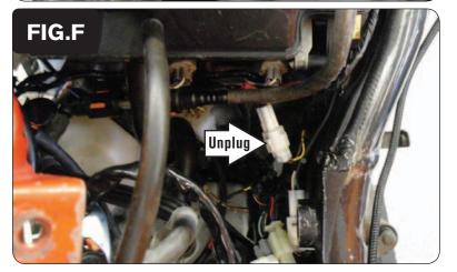
8 Locate and unplug the pair of stock Throttle Position Sensor connectors behind the throttle bodies on the right-hand side of the bike (Fig. F).
