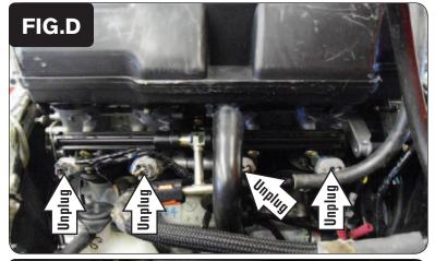
6 Unplug the stock wiring harness from the LOWER fuel injectors at the throttle bodies (Fig. D).
