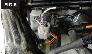
Plug the PCV connectors in-line of the stock wiring harness and the fuel injectors (Fig. E).
