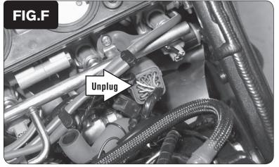
9 Locate and unplug the stock sub-harness connector for the bike's fuel injectors (Fig. F).
