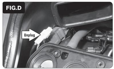
7 Locate and unplug the Throttle Position Sensor connector (Fig. D).
