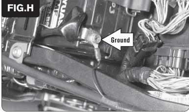
Secure the ground wire of the PCV wiring harness with the ring lug to the negative (-) terminal of the bike's battery (Fig. H).
