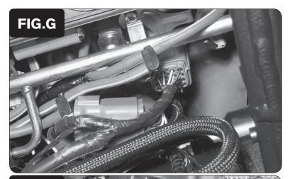
10 Plug the pair of 16-pin connectors of the PCV wiring harness in-line of the stock connectors (Fig. G).
