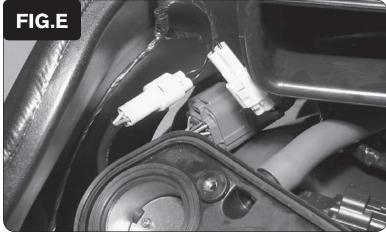
Plug the matching pair of WHITE 3-pin connectors on the PCV wiring harness in-line of the stock TPS connectors (Fig. E).
