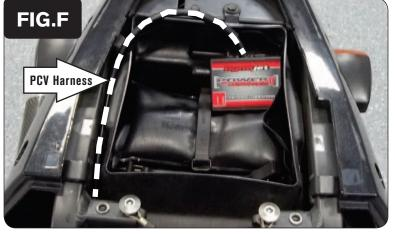
11 Secure the PCV module inside of the tail section (Fig. F).
