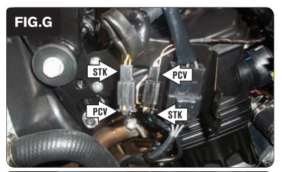
Plug the PCV in-line of the stock wiring harness and the Crank Position Sensor (Fig. G).
