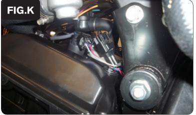
17 Plug the PCV wiring harness leads with BLUE colored wires in-line of the stock wiring harness and the right ignition coil stick (coil stick #2) (Fig. K).
