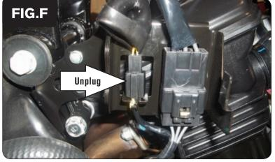
Locate and unplug the Crank Position Sensor from the stock wiring harness (Fig. F).
