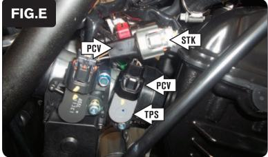
11 Plug the connectors from the PCV wiring harness in-line of the TPS and the stock wiring harness (Fig. E).
