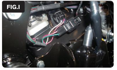
Plug the PCV wiring harness leads with GREEN colored wires in-line of the stock wiring harness and the left ignition coil stick (coil stick #1) (Fig. I).
