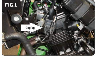
18 Locate the stock O2 sensor connection and unplug it (Fig. L)
