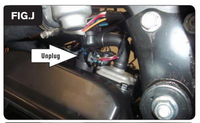
16 Unplug the stock wiring harness from the right ignition coil stick (coil stick #2) (Fig. J).
