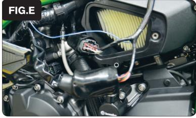
7 Plug the PCV in-line of the stock wiring harness (Fig. E).
