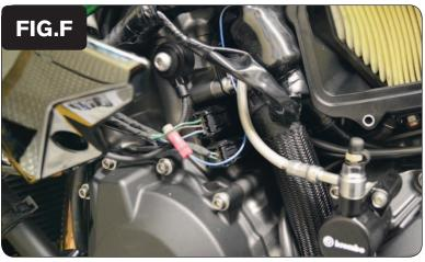
8 Using the supplied Posi-tap attach the BLUE/WHITE wire of the PCV to the stock GREEN/RED wire of the bike's Gear Position Sensor (Fig. F).
