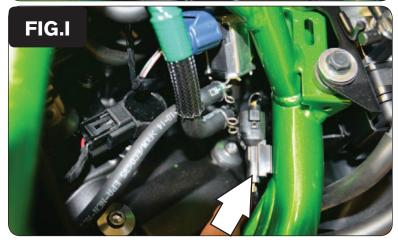
11 Unplug the crank position sensor connector (Fig. I).
