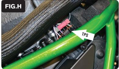
10 Using the supplied Posi-tap attach the GREY wire of the PCV to the stock PURPLE wire of the bike's Throttle Position Sensor (Fig. H).
