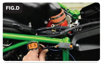
6 Route the PCV harness in-side of the frame (Fig. D)
