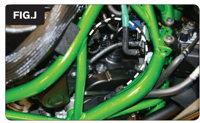
12 Plug the PCV in-line of the stock CPS and wiring harness (Fig. J).
