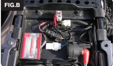
Attach the PCV module to the tray under the seat in the location shown in Figure B.
