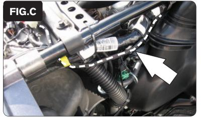
Route the PCV wire harness under the plastic tray and down the right hand side of the ATV, following the stock wiring harness (Fig. C).
