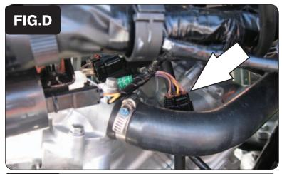
4 Locate the 6-pin BLACK connector on the front head, that comes from the throttle bodies. Unplug this connector (Fig. D).
