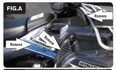
Remove the seat. Remove the right hand side cover, and the cover in front of the steering stem that holds the accessory outlet (Fig. A).
