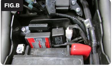
3 Secure the PCV module under the seat and next to the battery (Fig. B).
