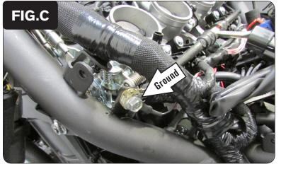
Secure the PCV ground wire with the small ring lug to the common ground location on the left side of the frame (Fig. C).
