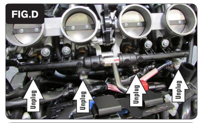
6 Unplug all four of the bike's Fuel Injectors (Fig. D).
