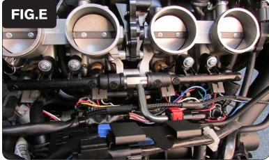
7 Plug the PCV wiring harness in-line of each injector and the stock wiring harness (Fig. E).
