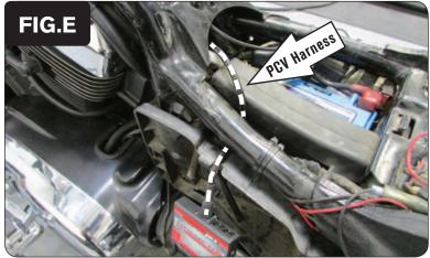
Route the PCV wiring harness between the plastic tray and the left frame rail (Fig. E). Continue routing beneath the frame/lower fuel tank mount and towards the throttle body.
