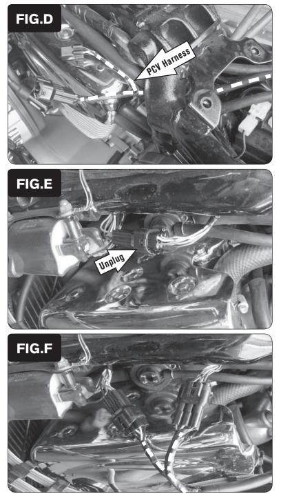
6 Continue routing the PCV wiring harness towards the front of the bike. Route underneath the frame and towards the left hand side of the rear cylinder (Fig. D).
